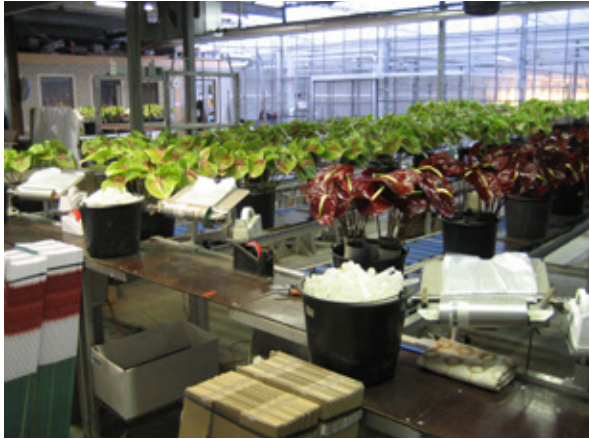
Buffer of roller tracks seen from the packing table
